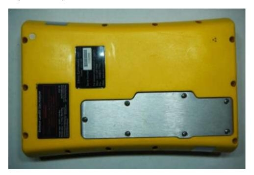
Remove the aluminum filter door by loosening the screws and lifting the door off of the enclosure. Warning: do not remove the filter door in dusty or wet atmospheres as the internal components can get damaged.
