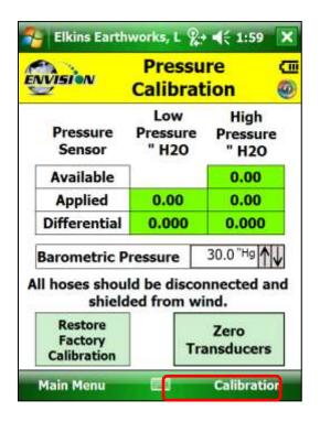
The pressure sensor calibration menu is also accessible from the pressure measurement screen in the analyze portion of the software. On the read "Pressures" screen tap the "Calibrate Sensors" button. This action will take you to the pressure sensor calibration screen that was just described in the previous section.
