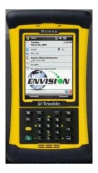
The Trimble handheld computer is the prime driver for the Envision® gas analyzer. The Trimble handheld computer, provided with the Envision® gas analyzer package, has already been prepared for field use. A screen protector has already been applied to your Trimble unit. An extra screen protector has been included in the packaging.
