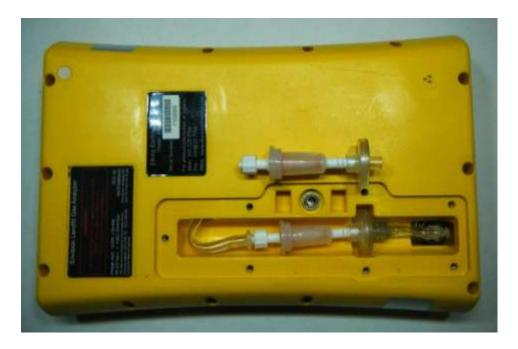
The user may now remove and replace the filters by turning the Luer filter fittings. Make sure the seal is still in place and re-attach the filter door. Replacement Luer filters may be purchased from Elkins Earthworks®.
