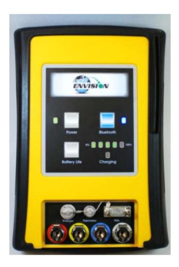
The Envision® gas analyzer houses the gas and pressure sensors. The gas analyzer utilizes infrared sensors to measure  $CH_4$  and  $CO_2$ . The Envision® uses an electrochemical cell to measure  $O_2$  concentration and an accurate thermistor temperature probe to measure wellhead gas temperatures. Data generated by the Envision® gas analyzer is relayed to the Trimble® via Bluetooth or serial cable several times per second.
