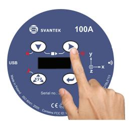
5) Start the calibrator using level of 1 m/s<sup>2</sup> at 16 Hz and wait until all 3 LEDs are green.
