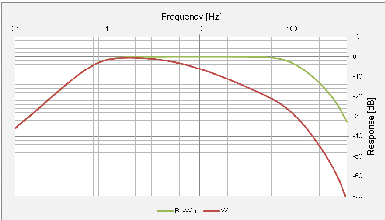
Characteristics of the BL-Wm and Wm digital filter implemented in the instrument
