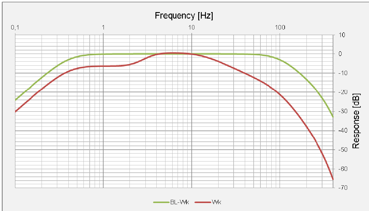
Characteristics of the BL-Wk and Wk digital filters implemented in the instrument
