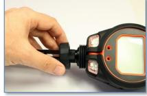
2. Remove the filter clamp and tube holder together.
