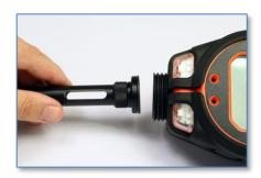
3. Place the O-ring on the filter lamp and push the assembly in to the filter housing with the window facing forward. Continual pressure may be required to keep the assembly in place while tightening the filter cap.
