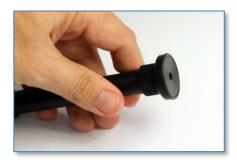
The filter disk should be replaced if it appears dirty, or is disturbed from its seating position.
