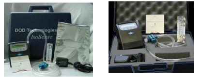
The IsoSense sampling unit has a digital display which displays battery life, flow rate and sample time. This smart sampling unit will constantly checking for restricted air flow, blocked airflow or over flow while automatically adjusting and maintaining the preset value.
