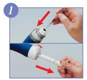
Insert <u>a sealed</u>, <u>unbroken detector</u> <u>tube</u> into the rubber tube connector. Align the red line on the bottom case and that of shaft, and pull the handle to full stroke locked position.
