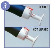
Wait one minute. Unlock the handle by turning it 1/4 turn (90 degrees), and check to see if the handle returns to the initial position. When the lock is released under full vacuum, the handle tends to snap back quickly. To prevent possible damage to the locking device allow the handle to return slowly by holding the cylinder and handle securely. If the handle returns completely to the original position, the performance is satisfactory.
