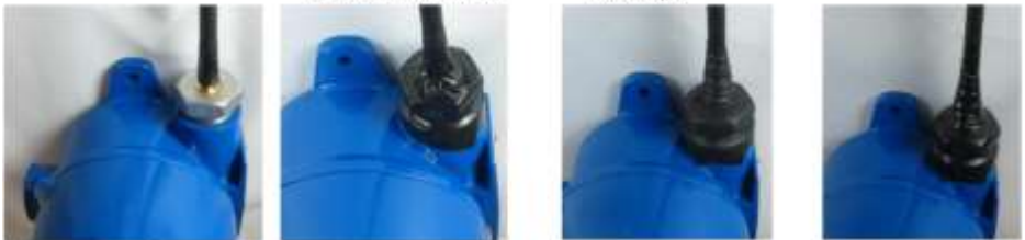
Figure 2-9: Water Proofing Antenna Connections
