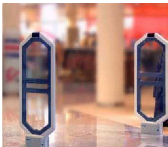
Magneto acoustic gate used for product surveillance
