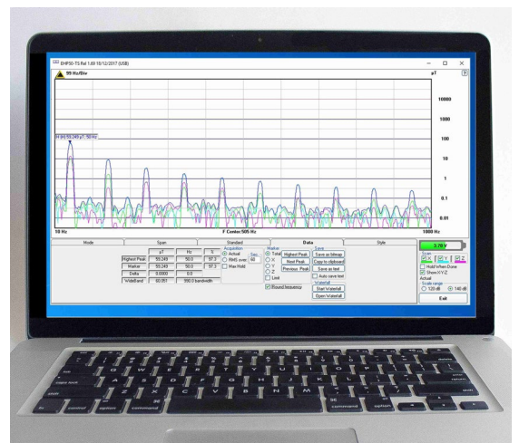
Measurement controlled by PC with EHP50-TS
