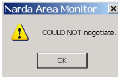
GSM Communication error. Maybe there is too much traffic on the base station that is communicating with 2600 or the SIM card is not enable for data exchange.
