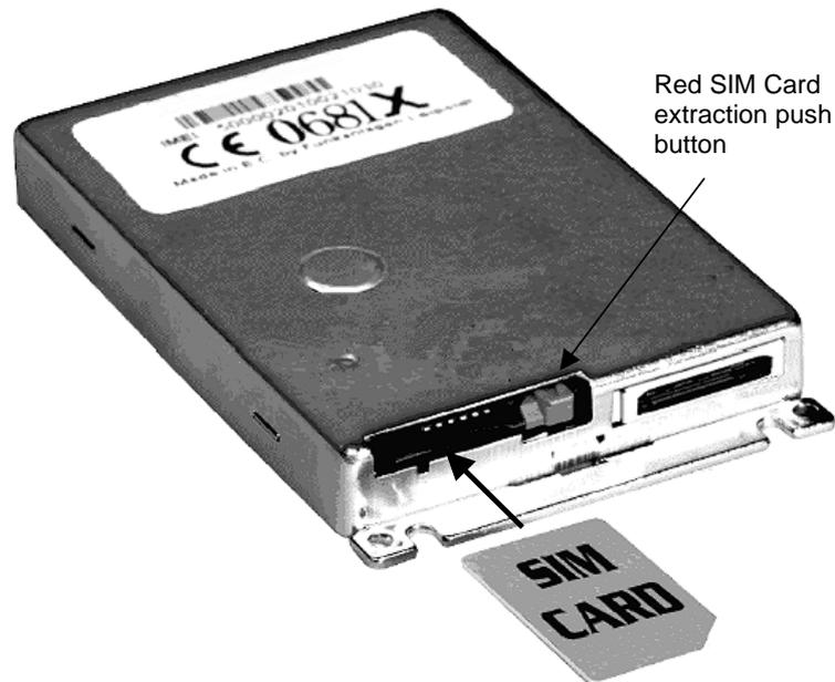
The modem is located on the lower part of the equipment, near the probe connector, the SIM CARD must be inserted in the slot like in the above figure, to extract it use the red push button.
