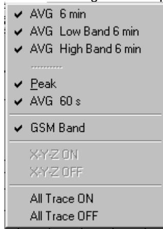
Since EP-3TB does not provide X, Y and Z axis, this function is disabled.
