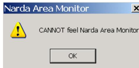
The station does not answer. 2600 could be OFF or the internal GSM is OFF or the battery is below the minimum value.
