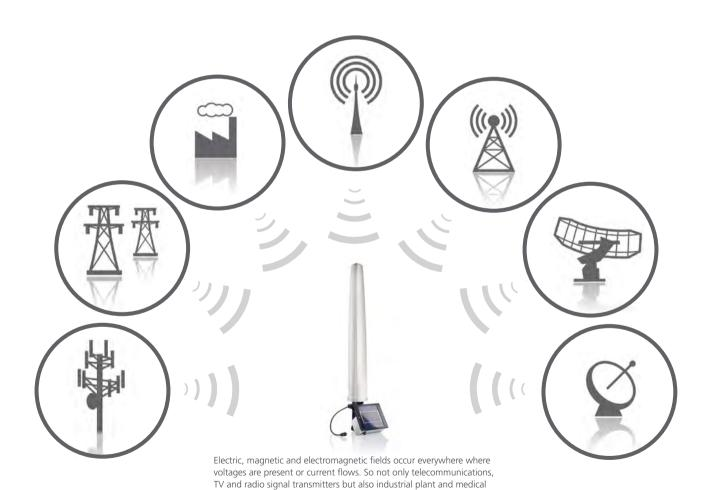
equipment emit electromagnetic fields. This is sometimes the desired effect, as in telecommunications for transmitting information, and at other times it is an unwanted side effect – from high voltage cables, for example.
