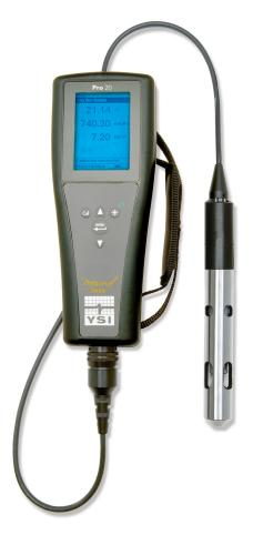
Parameters: Dissolved Oxygen % and mg/L (electrochemical) Temperature BOD (biochemical oxygen demand)
