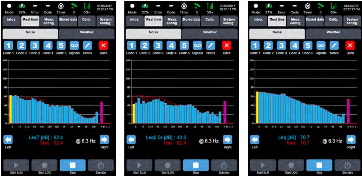
LeqT: equivalent continuous level calculated over the logging period
