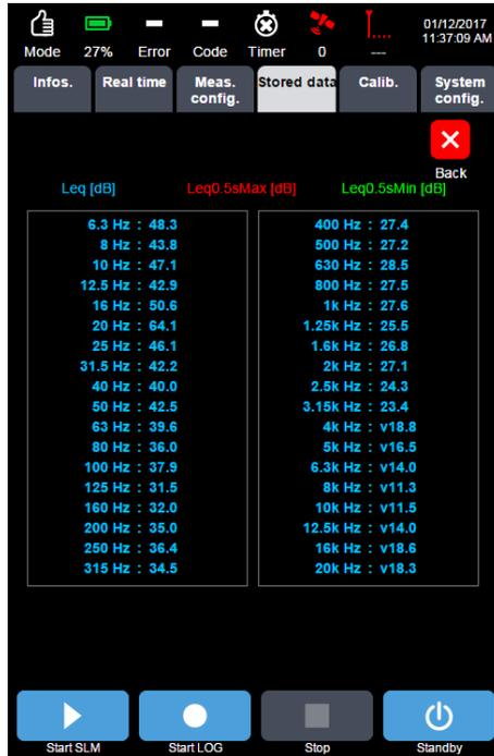
Max./Min. values can be displayed by selecting the indicator in red for Max values or green for Min. values.
