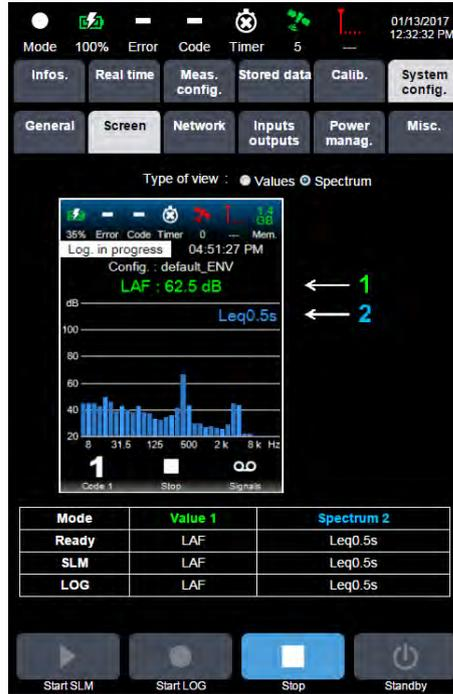
Internal display example for spectrum
