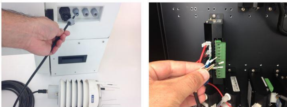
Figure 0-12 To connect third party sensors such as weather sensors, feed the cable through the gland and wire to the green plug.
