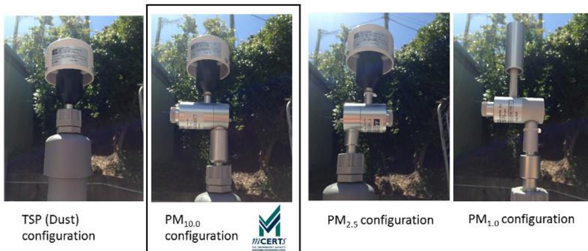
Figure 0-12 Size selection in the Particle Monitor is determined by the sharp cut cyclone on the inlet
