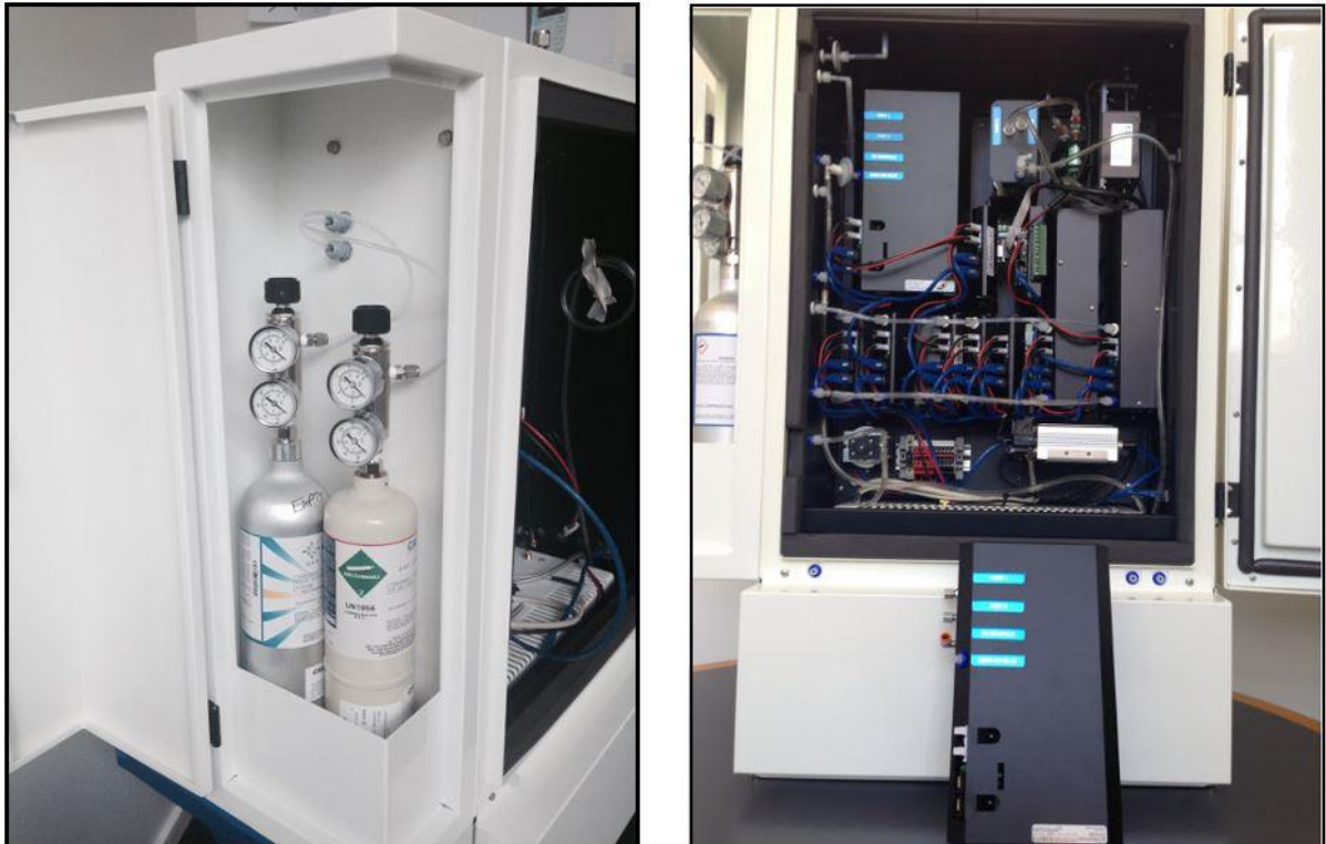
Figure 0-5 The AirCal 8000 stores calibration cylinders in a compartment on the left side. All of the components required to perform the calibration are in a module inside the AQM 65.
