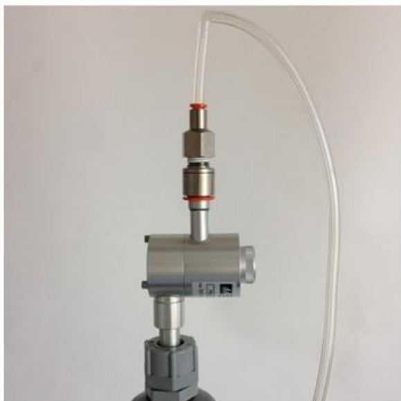
Figure 0-15 When checking the flow rate of the Particle Monitor (left) place the flow measurement adaptor above the cyclone. The position of the flow adaptor when measuring the Particle Profiler is shown on the right.
