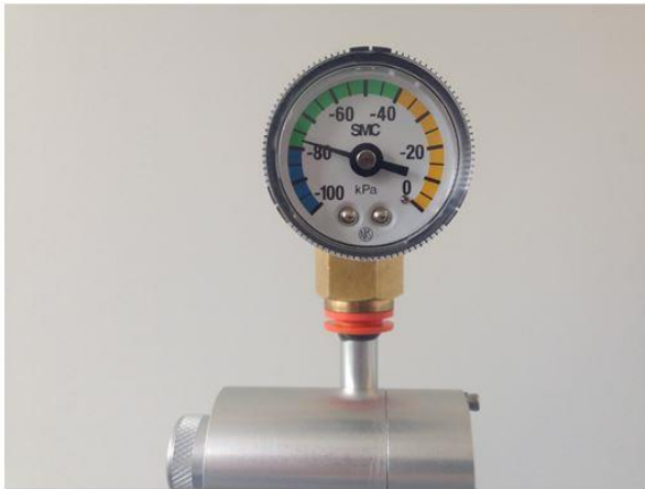
Place gauge on inlet above cyclone
