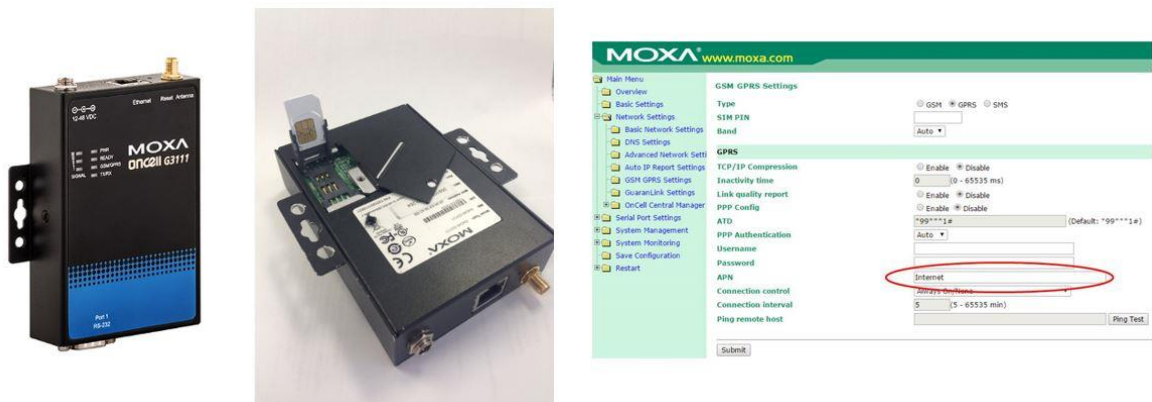
Figure 0-13 A SIM card must be inserted in to the modem and the Modem must be configured
