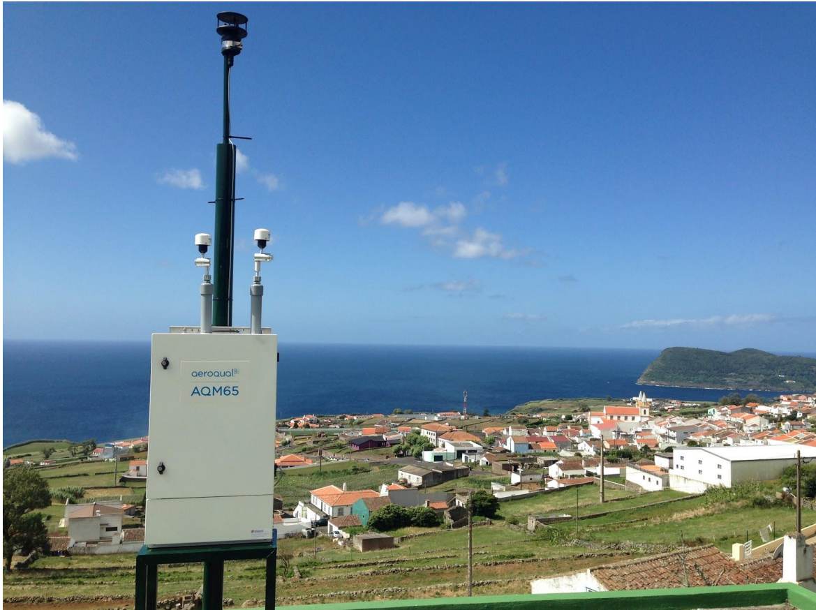
Figure 1: The AQM 65 is mounted on a stand and is secured to a pole. A wind sensor (Gill) is mounted to the top of the pole.
