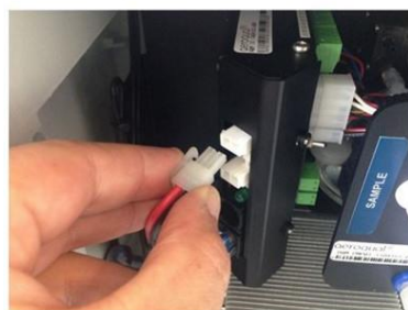
Figure 0-19 Fit the vacuum gauge, adjust the valves. Then stop the pump by removing power from the module, observe the change in pressure. If the leak rate is greater than 10 kPa in 10 seconds then there may be a leak in the system. Check all the tube connections.
