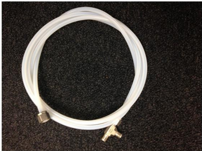
Figure 0-6 The AQM CALKIT connects the output of the AirCal 1000 to the input of the AQM 65 via a tee.
