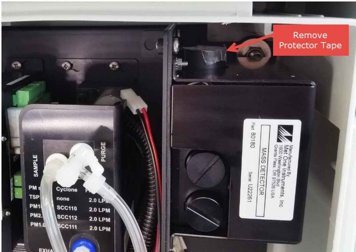
Figure 0-5 Remove the protective tape from the PM inlet
