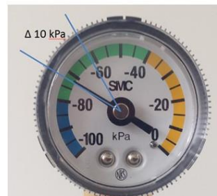
Figure 0-19 Fit the vacuum gauge, adjust the valves. Then stop the pump by removing power from the module, observe the change in pressure. If the leak rate is greater than 10 kPa in 10 seconds then there may be a leak in the system. Check all the tube connections.
