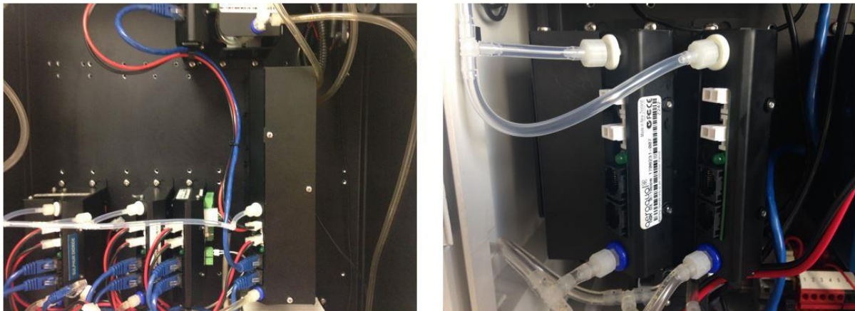
Figure 0-6 Left: The large size direct NO 2 measurement module, Right: Ox/O 3 system for measuring NO 2
