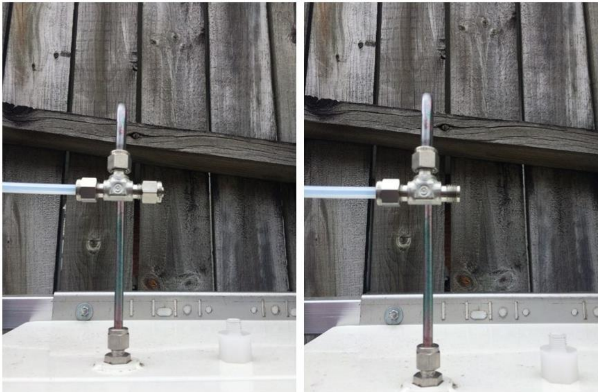
Figure 0-2 Left: Closed tee used with demand flow regulator. Right: Open tee used with fixed flow regulator.
