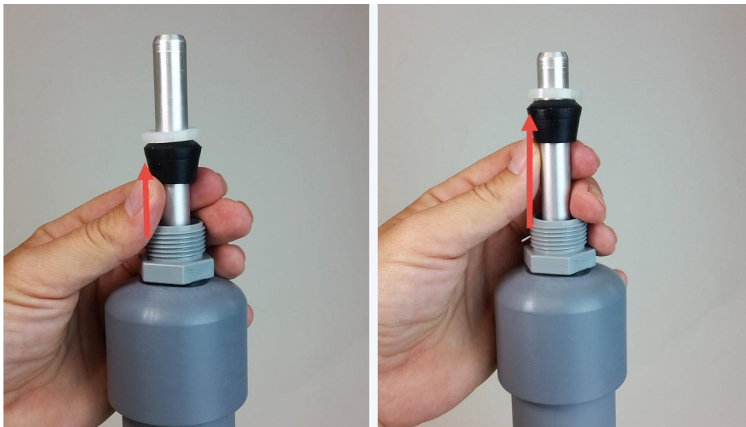
Figure 0-8 Create more length to the inlet by sliding the black rubber grommet up the tube.
