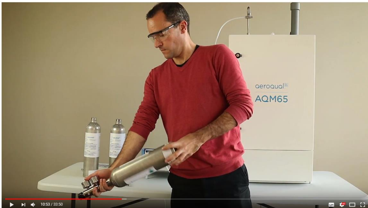
Figure 0-9 Calibration of Ox Ozone system for NO 2 YouTube: www.youtube.com/watch?v=InK1x7mTTQw
