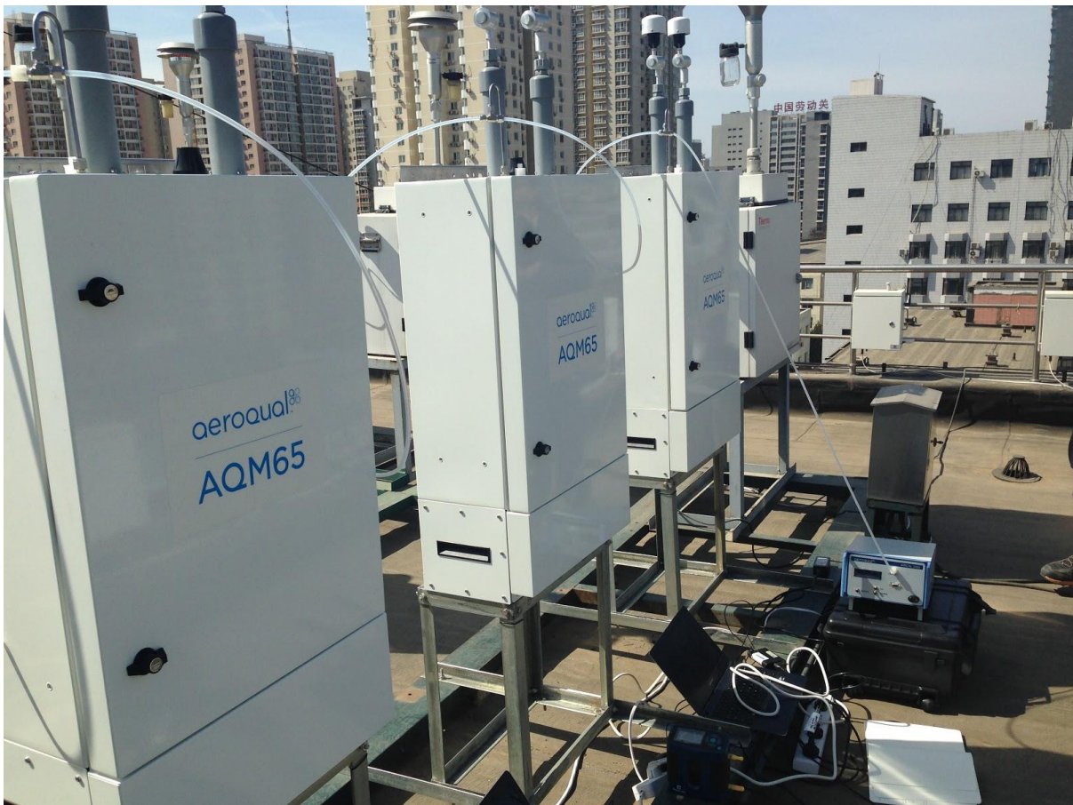
Figure 0-4 The Ozone calibrator and AirCal 1000 can calibrate multiple instruments at the same time.
