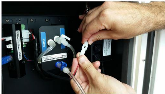
Figure 0-10 During field installation, secure the PM inlet using the retaining screws and plug in the heater
