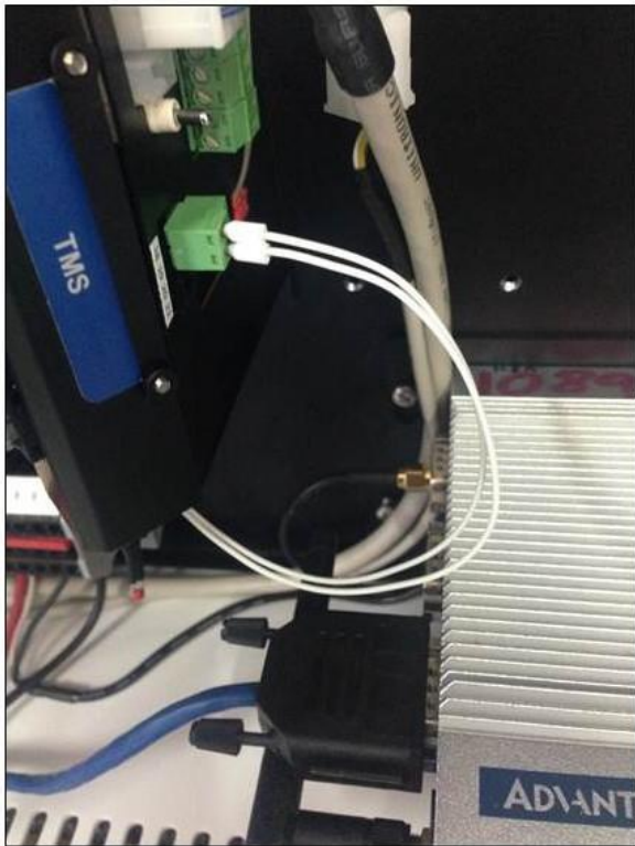
Figure 0-35 Replace the internal temperature sensor with the temporary plug shown
