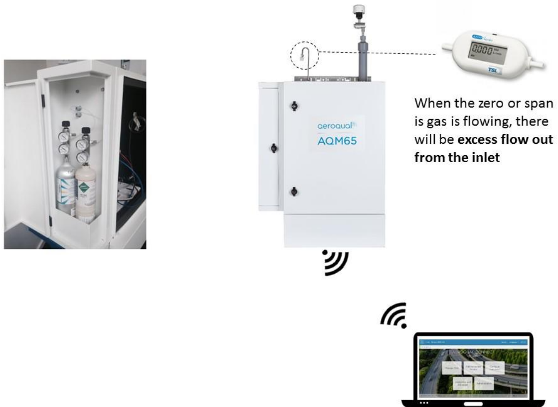
Figure 0-14 Setup to perform a zero and span calibration using the AirCal 8000
