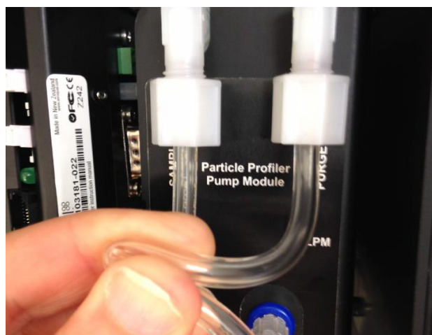
Figure 0-21 Pinch the tube with the newer pump module
