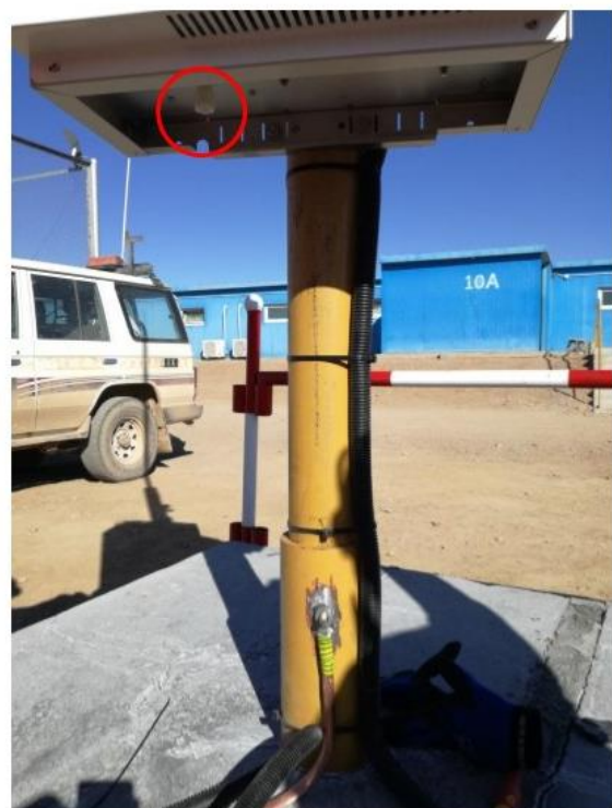
Figure 2: It is very important to maintain good air flow underneath the AQM 65. The temperature and relative humidity sensor is placed on the bottom plate (right) The AQM 65 should be mounted on an open bottom stand so that air can flow underneath the AQM 65, the cooling fan at the back (left) must also be unobstructed.
