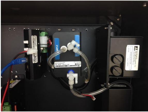
Figure 0-4 With mains power on, and with the 12 V DC fuse pulled out, there should be air flow coming from the top of the AQM as shown on the right. Disconnect the power (red/back) cable from the PM pump module while testing the power, as shown on the left
