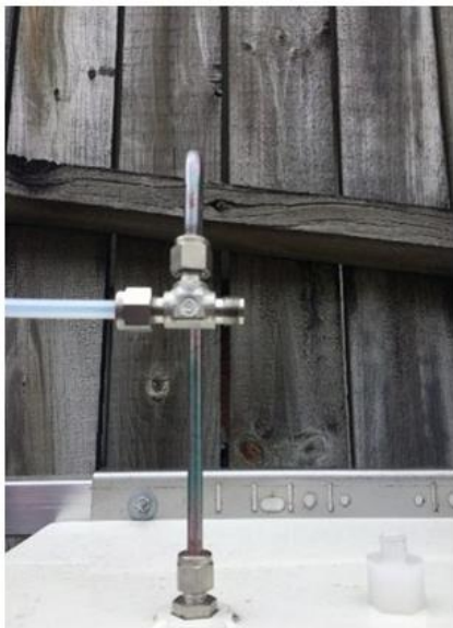
Figure 0-6 The AQM CALKIT connects the output of the AirCal 1000 to the input of the AQM 65 via a tee.
