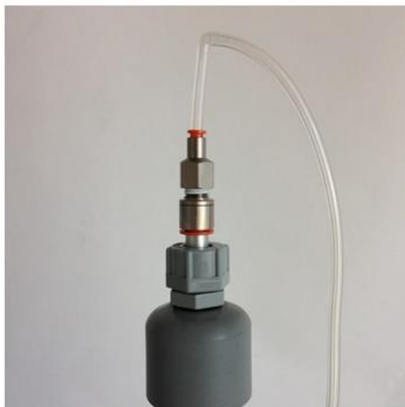
Figure 0-15 When checking the flow rate of the Particle Monitor (left) place the flow measurement adaptor above the cyclone. The position of the flow adaptor when measuring the Particle Profiler is shown on the right.
