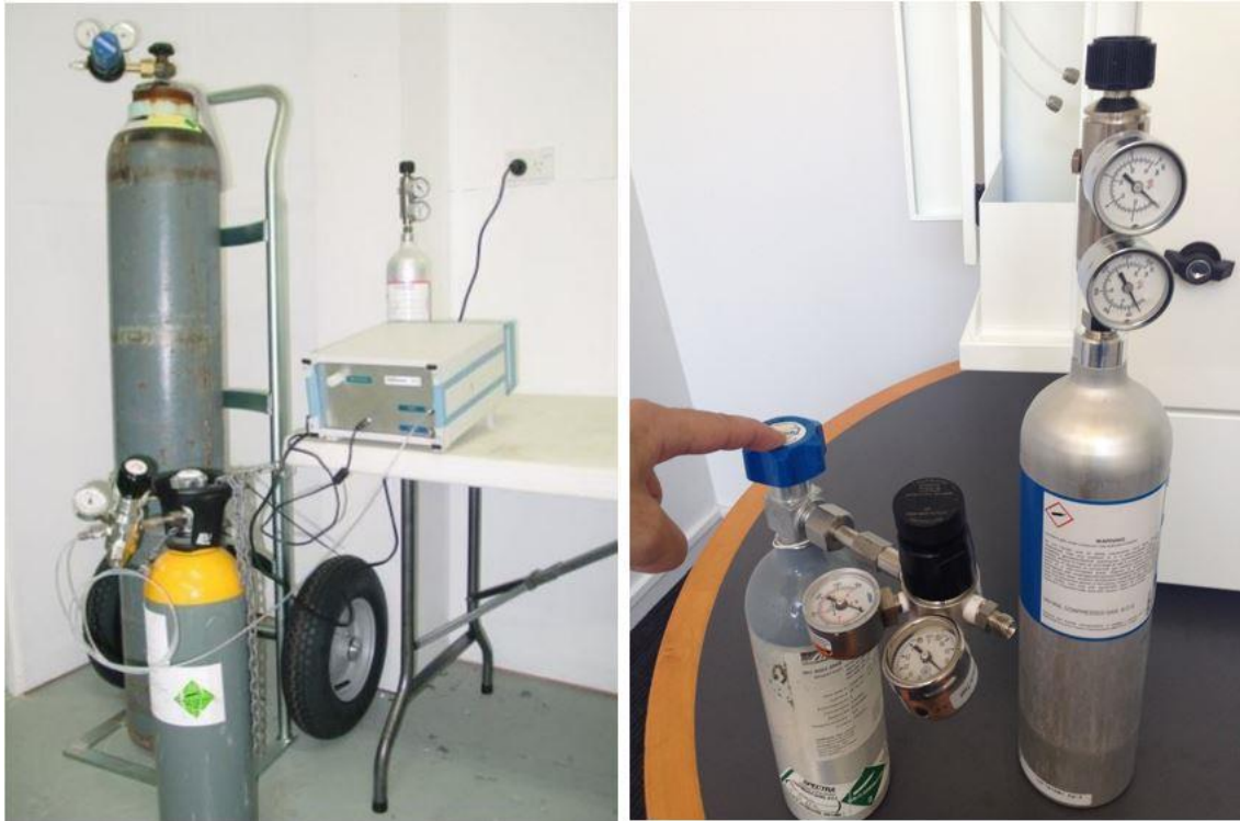
Figure 0-1 The left side image shows a large and medium laboratory gas cylinder. Both can be used with the AirCal 1000 or AirCal 8000. On the right-hand side are small size cylinders from Linde and Calgaz. These are more convenient and easier to transport.
