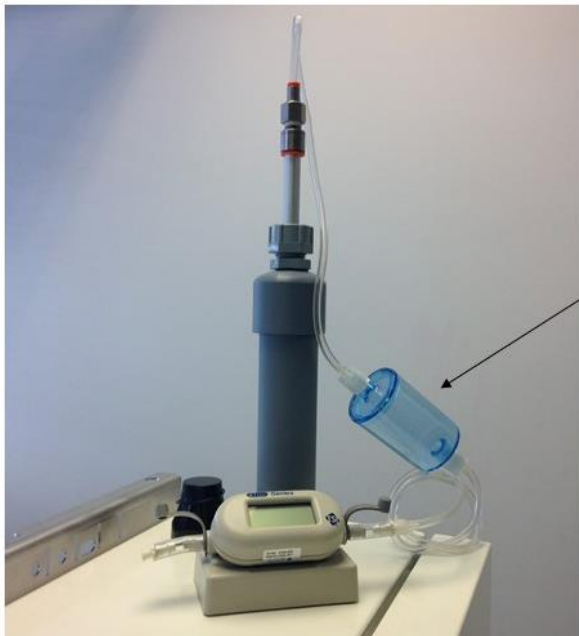
Figure 0-17 When measuring the flow on the Particle Profiler it is important to use the flow buffer chamber
