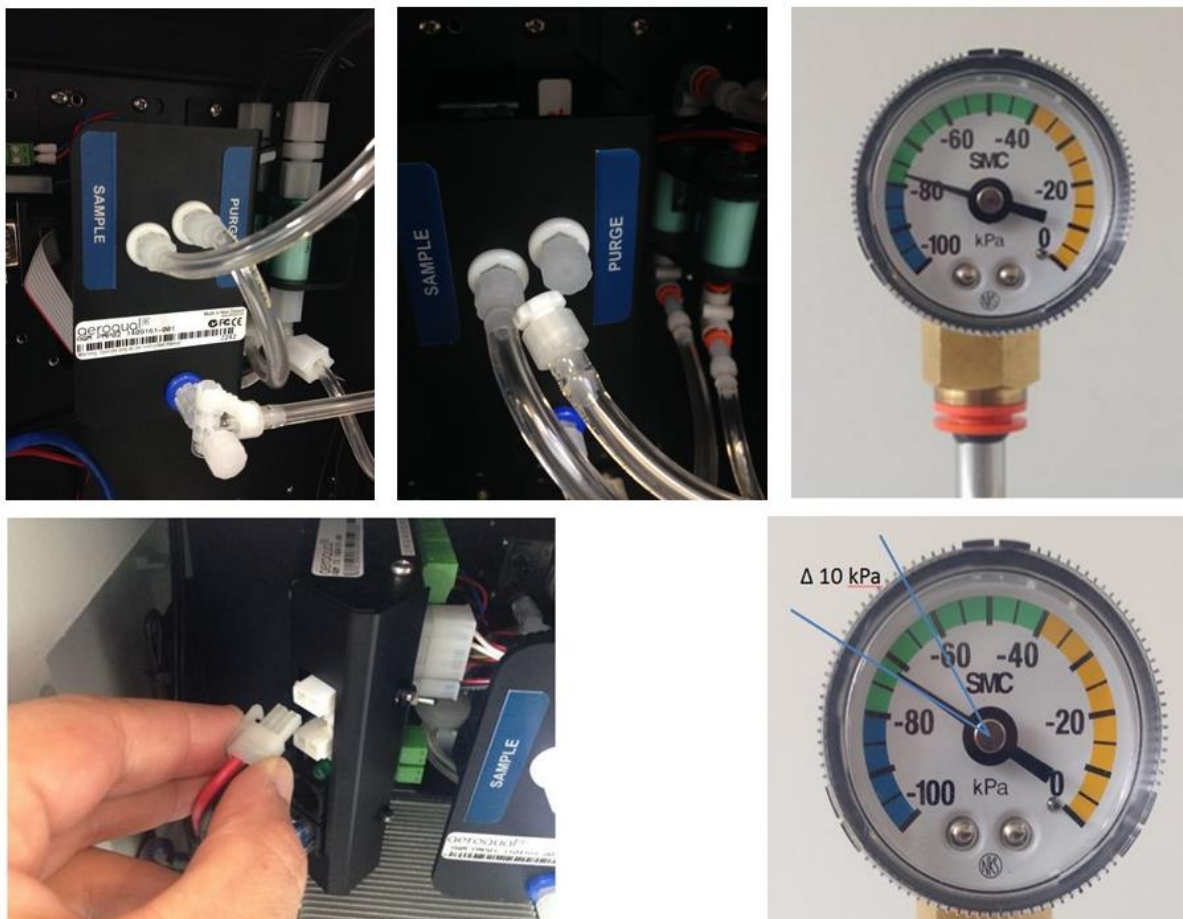
Figure 0-20 Cap the purge and exhaust lines. Place the vacuum gauge on the inlet. Disconnect the power, observe the change in pressure.
