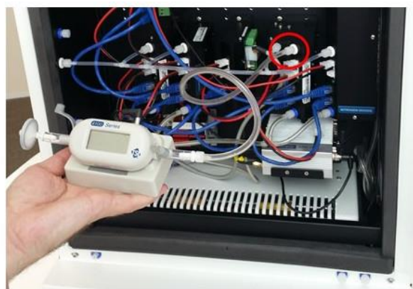
Figure 0-7 To measure the individual module flow rates, disconnect the gas inlet and attach the module inlet to the vacuum port of the R7 flow meter.
