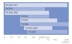
Conductivity Cell Selection Chart for the 3200 (For the 3100 see specific ranges on back)
