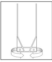
Fold the two holes at bottom of HydraSleeve together and attach weight
