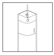
Attach line to hole at top of HydraSleeve.
