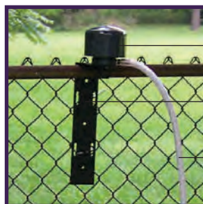
Rain cover protects sampling head
