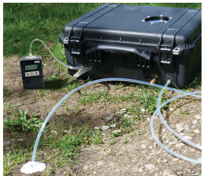
Vac-U-Chamber in use with AirChek XR5000 Sample Pump
