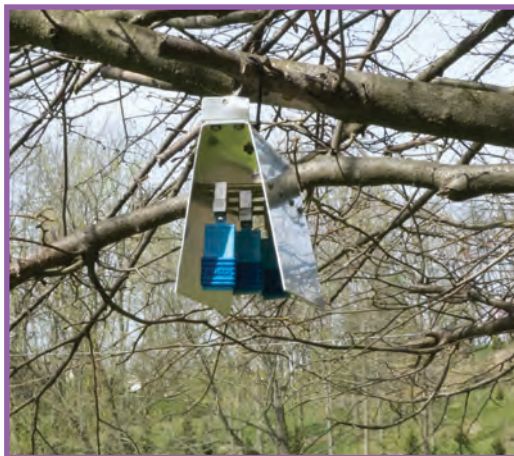
Outdoor sampling shelter protects multiple samplers.
