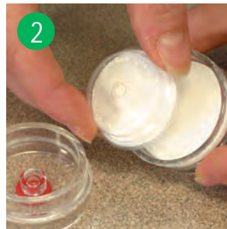
2 Weigh Accu-CAP and insert in cassette.
