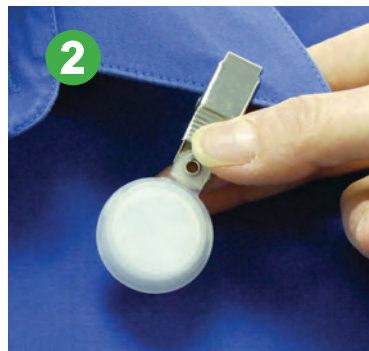
Clip in worker's breathing zone to sample.
