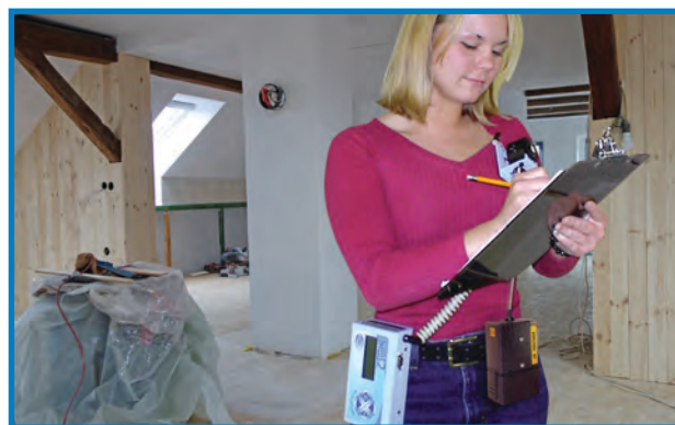
Attach to a pump to monitor dust levels in real time while collecting a gravimetric sample. SKC recommends using the AirChek 52/Sidekick pump. See pages 12-13.
