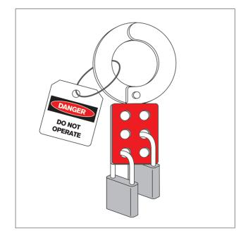
Figure 3 – Example of tag and lockout with the padlocks of two employees
