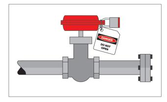
Figure 4 – Open end of pipe capped. Nearest valve closed, locked and tagged
