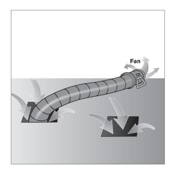
Figure 8 – Local exhaust ventilation
