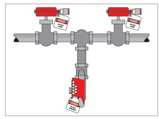
Figure 6 – Closing, locking and tagging at least two valves in the piping leading to the confined space. Drain valve locked open to atmosphere and tagged
