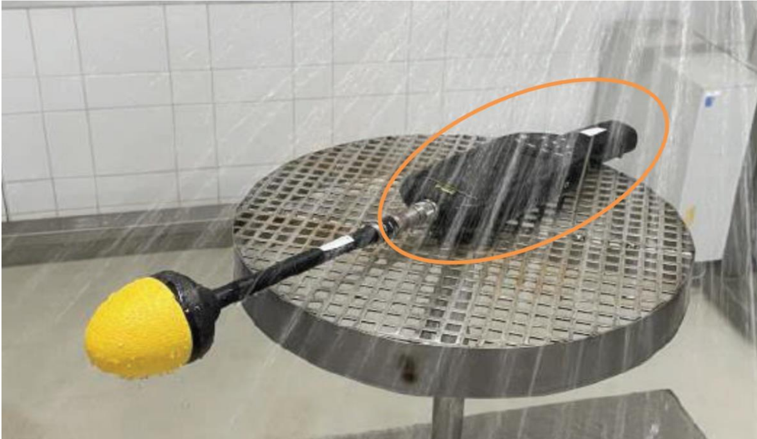
Type approval test for IP 54 (splash-proof)
