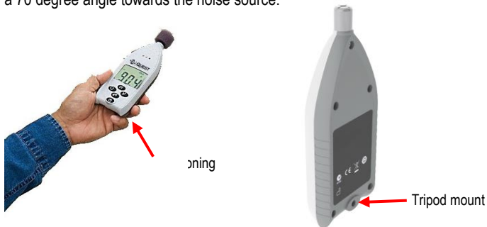
Figure 1-9: Positioning and tripod mount
