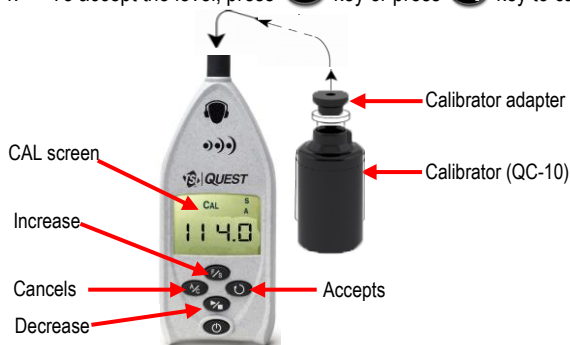
Figure 1-10: Calibrating the SD-200
