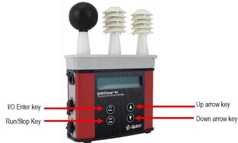
Figure 1-2: Keypad explained and identified
