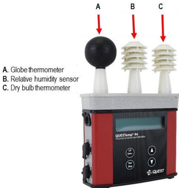
Figure 1-5: Sensors identified
