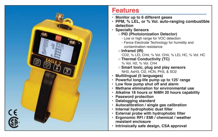
RKI is proud to offer the next generation of our popular EAGLE portable gas detector. Equipped with features that are not available on competitive units, the EAGLE 2 is a powerful instrument that does more than just offer the standard confined space protection for LEL, O2, H2S and CO.
