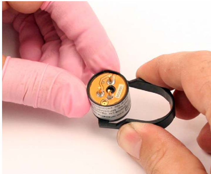
Figure 29: Using Removal Tool
