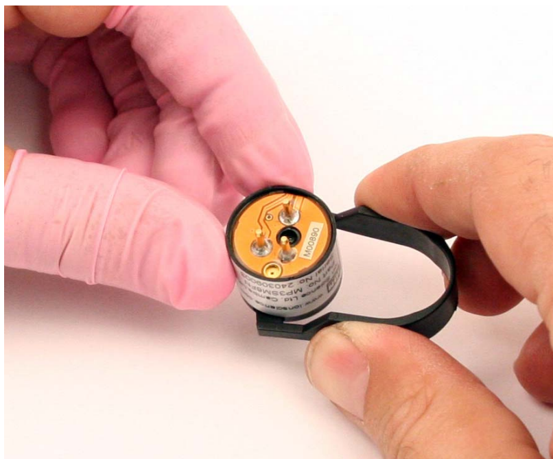
Figure 33: Using Removal Tool
