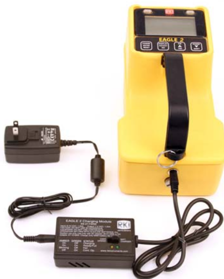
Figure 17: Connecting the EAGLE 2 to the Charger
