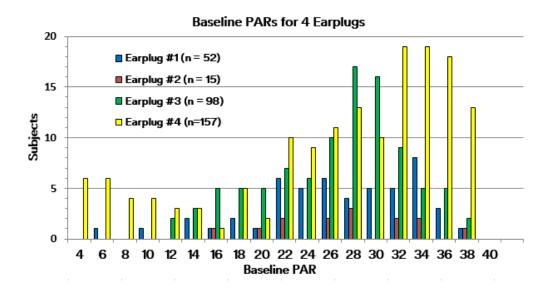
Figure 1 – Initial baseline PAR measurements of 4 earplugs for a group of manufacturing workers (n=322).
