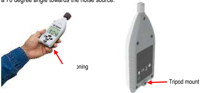
Figure 1-9: Positioning and tripod mount
