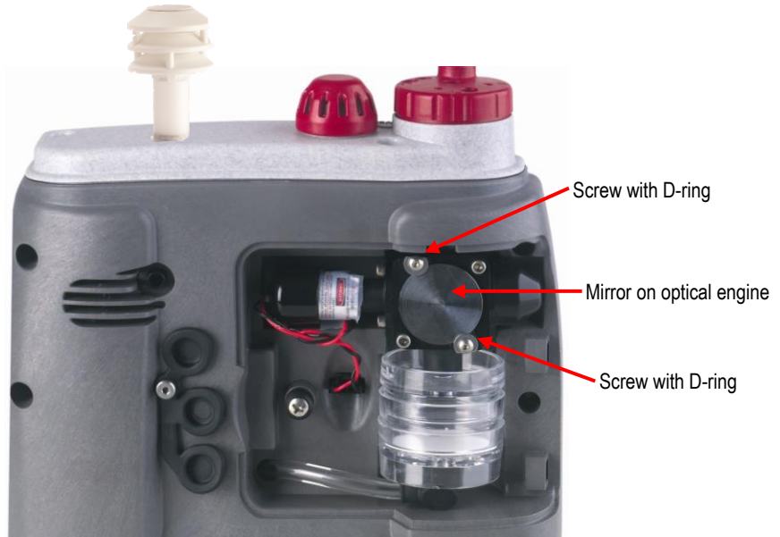
Figure 7-7: Optical engine and cleaning
