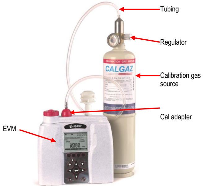
Figure 4-17: Applying a gas sensor
