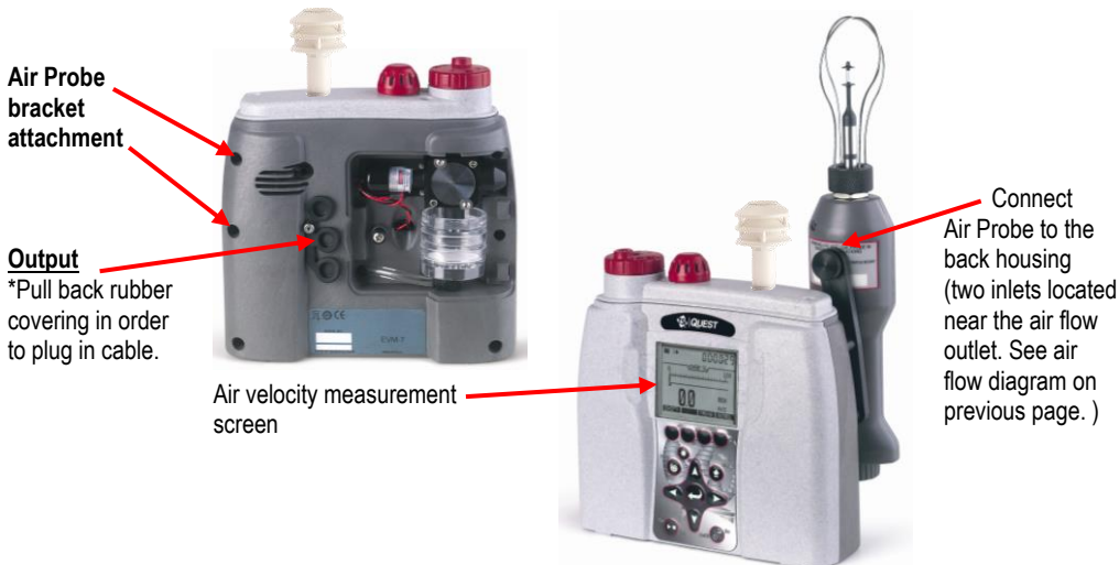
Figure 5-11: Attaching Air Probe and measuring Air velocity
